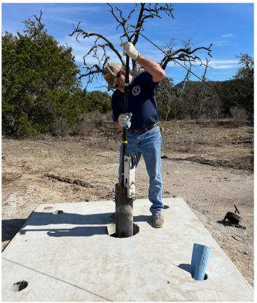
L. Thomas conducting a geophysical log; lifting the logging probe out of the wellhead.
