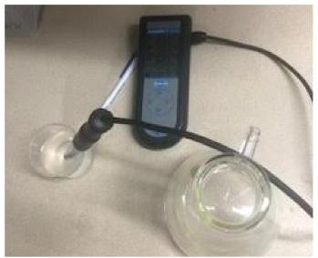
Probe used to read a water's pH level in the BCRAGD lab.
