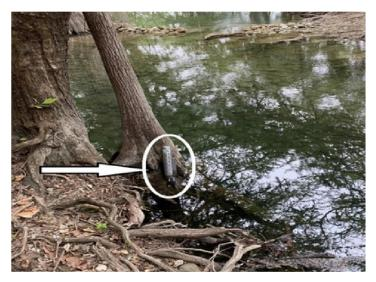
One of Five USGS Insitu Pressure Transducer, Water Level Electronic Data Loggers – Installed Above Utopia, TX, along the Sabinal and West Sabinal River.
