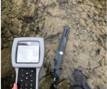
Sonde Meter – Water analysis tool used by BCRAGD for surface water quality monitoring.
