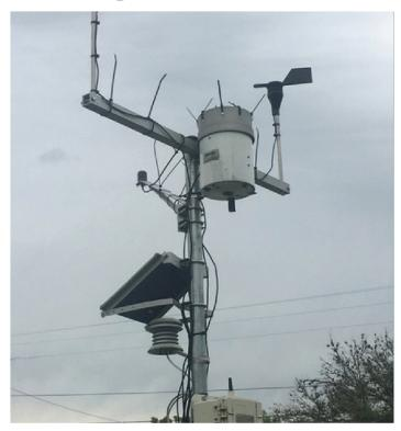
*The image above shows the EAA weather station and rain gage that provides information to the HOBOlink.*
