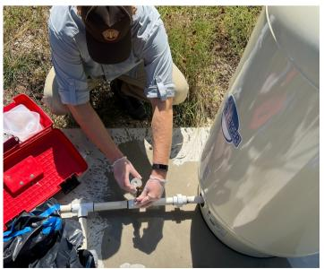
BCRAGD staff collecting a sample from a water well for a post drill inspection
