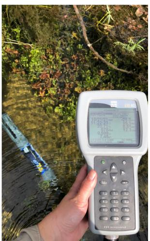
Sonde Meter being used to conduct surface water sampling
