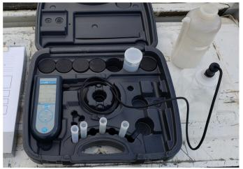
This photo shows the water-quality probe being used to test the water of a monitor well. Some of the measurements taken here were temperature, pH, conductivity, and total dissolved solids.
