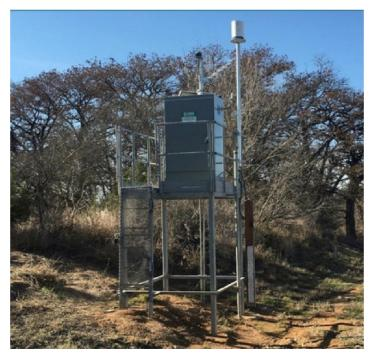
USGS Stream Gage at Sabinal River Bridge at Utopia, TX FM-1050, 08197970 Sabinal Rv at Utopia, TX. The photo was taken on March 4, 2020. Stream Gage is located on the Left Bank-Downstream side of the bridge near the top of the stream bank.
