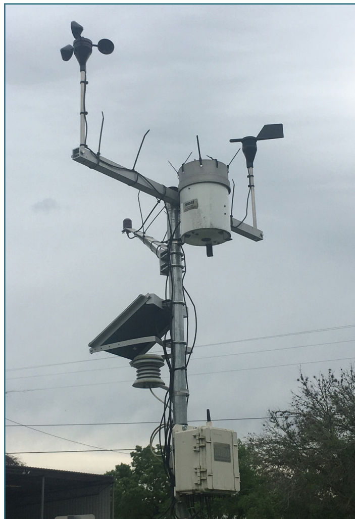
The image above shows the EAA weather station and rain gage that provides information to the HOBOLink.
