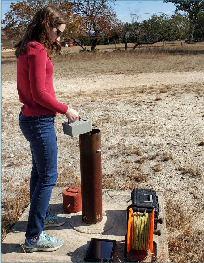
BCRAGD's Groundwater District Operations Manager, Alyssa Balzen, checking Monitor Well levels.
