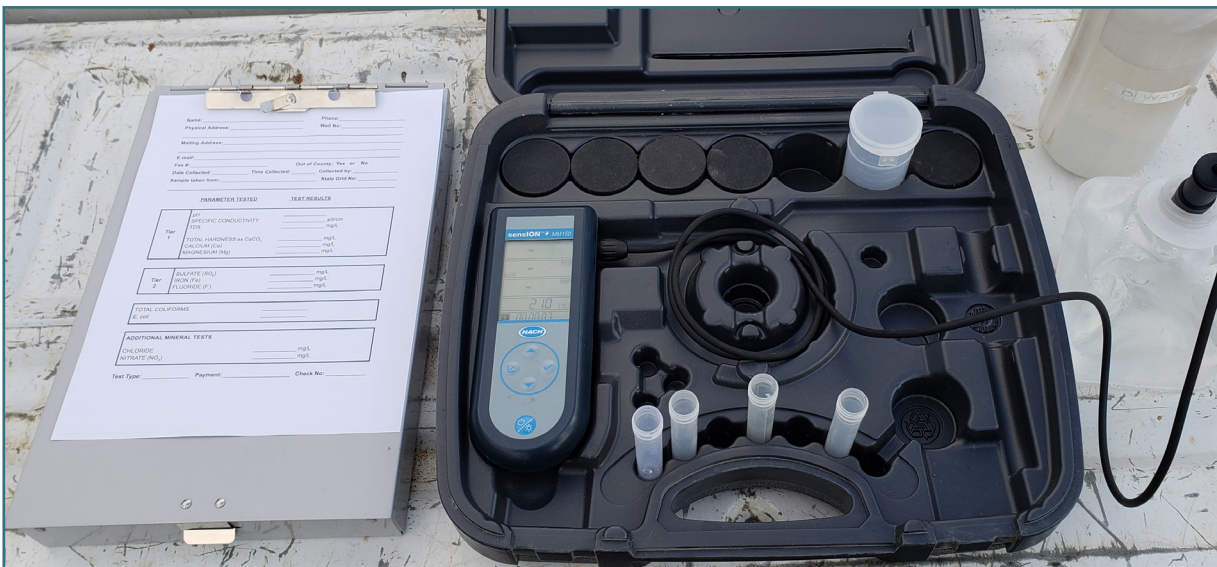
This photo shows BCRAGD staff analyzing the water quality of a Monitor Well using a probe while in the field. Some of the measurements taken here were temperature, pH, conductivity, and total dissolved solids.
