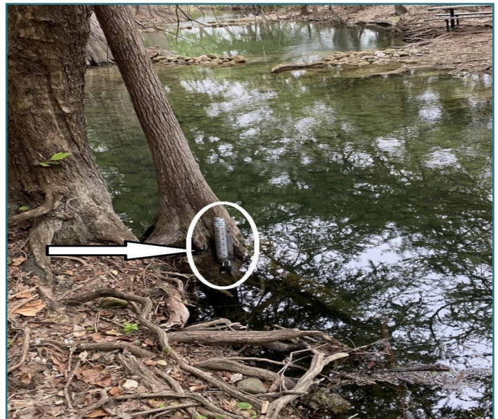
One of Five USGS Insitu Pressure Transducer, Water Level Electronic Data Loggers – Installed Above Utopia, TX, along the Sabinal and West Sabinal River.
