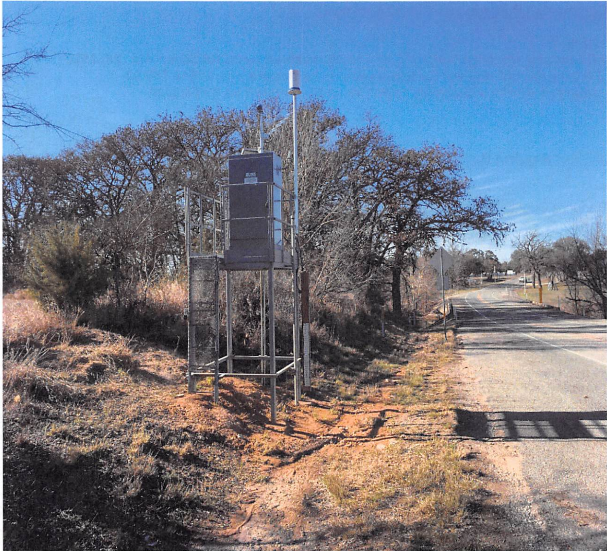
Newly installed USGS Stream Gage at Sabinal River Bridge At Utopia, Tx FM-1050
